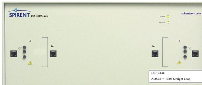
Figure 1.1 DLS 414E ADSL2++ Wireline Simulator
